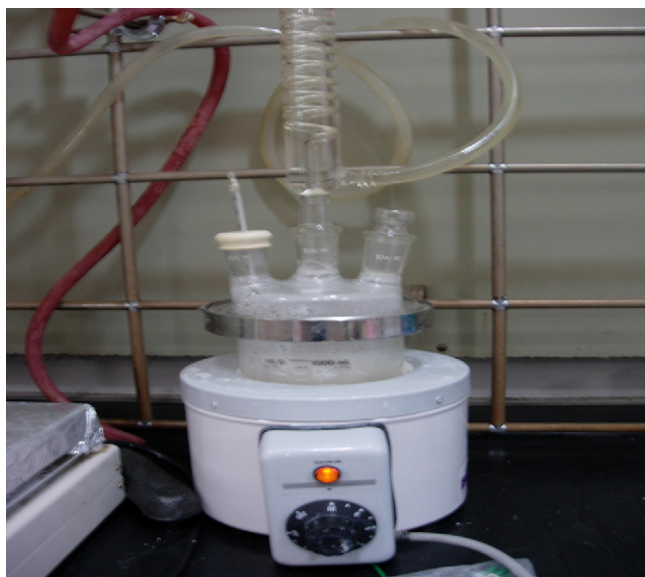
Fig. 1. A photograph of the reflux glass vessel for the production of high purity mesoporous silica from hexafluorosilicic acid as a waste material of phosphate fertilizer industry.
